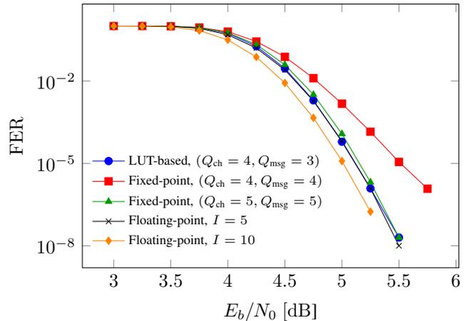
**Fig. 4:** FER vs  $E_b/N_0$  for the  $N = 2048$  (6, 32)-regular LDPC code defined in IEEE 802.3an.
