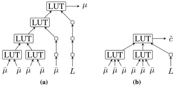
**Fig. 3:** (a) A variable node LUT tree for the calculation of one output of a variable node of degree  $d_v = 6$ . Each LUT-based variable node contains  $d_v$  such LUT trees, one for each of the  $\binom{d_v}{d_v-1}$  possible combinations of input messages.
