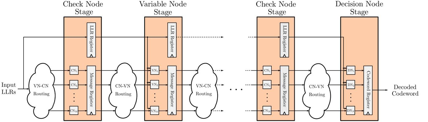
**Fig. 2:** Top level decoder architecture processing pipeline. The channel LLRs are the input of the left-hand side and the decoded codeword is obtained as the output of the right-hand side.
