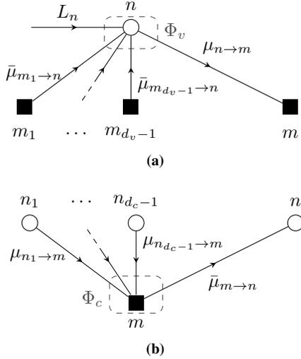
**Fig. 1:** VN update (a) and CN update (b) for  $\mathcal{N}(n) = \{m, m_1, \dots, m_{d_v-1}\}$  and  $\mathcal{N}(m) = \{n, n_1, \dots, n_{d_c-1}\}$
