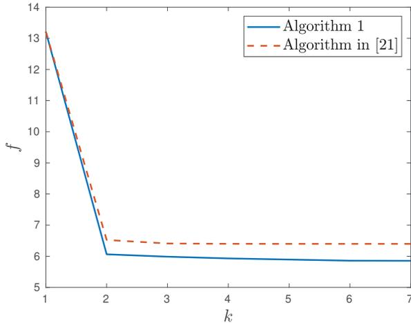
Fig. 7: Convergence process of the proposed PGD algorithm versus the LMI-based algorithm in [21].
