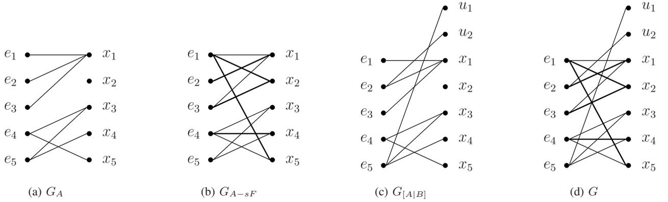
Fig. 2: Bipartite graph representation of descriptor system (1) with (5) and  $B_2$  in (6). The bold edges represent s-arcs.
