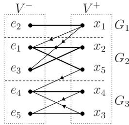
Fig. 3: DM decomposition of  $G_{A-sF}$  of descriptor system (1) with (5). The bold edges represent s-arcs.
