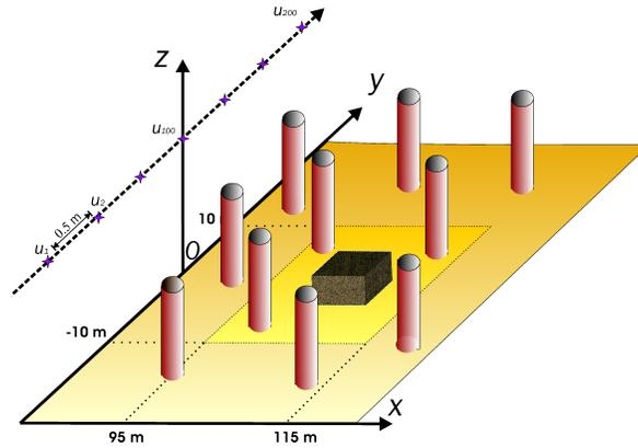
Fig. 6. Scene configuration for the simulated data. A PC box of size  $(2\text{m} \times 1.5\text{m} \times 1\text{m})$  over a PC flat ground and located at position  $(108, -1)\text{m}$  is placed in a forest of dielectric trunks, for an transmitted signal with center frequency of  $400\text{MHz}$  and with bandwidth of  $100\text{MHz}$ . The attenuation due to the canopy is also taken into account.
