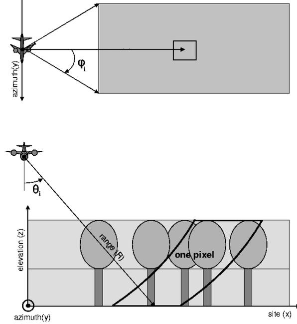
Fig. 2. Definition of the incidence angles  $(\theta_i, \varphi_i)$ .
