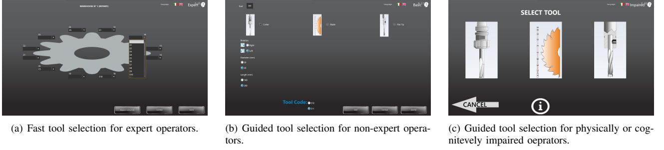
Fig. 4. Examples of an adaptive HMI for machine setup operations.
