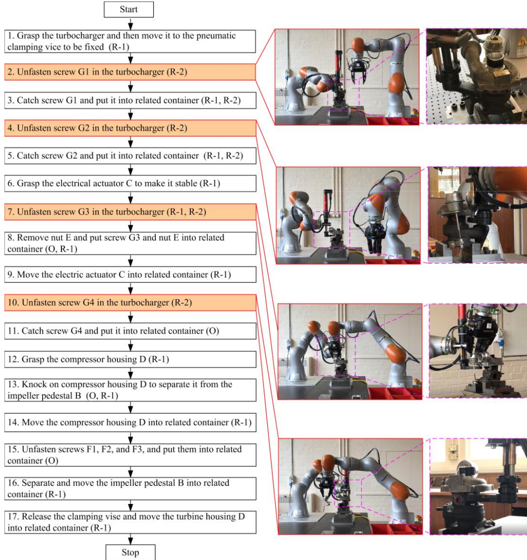
Fig. 19. Flowchart of the turbocharger disassembly operations.
