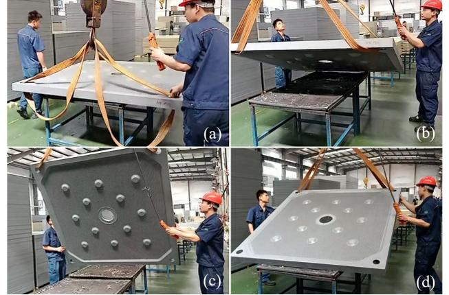
Fig. 1: Human workers in a sewage press machine factory flip press boards with the help of a gantry crane. (a) Attaching the board to the crane hook using bearing belts. (b) Activating the crane to lift up the board. (c) The board is lifted up to a satisfying pose. (d) The board is flipped and is returned to the workbench.
