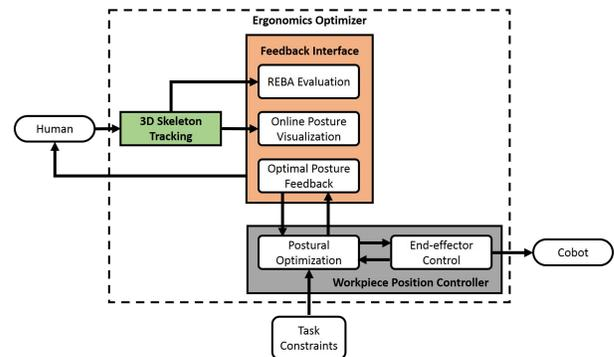
Fig. 5: Ergonomics controller scheme. Based on the ergonomics analysis and the task data (workpiece constraints) optimal postures are suggested to the user or the cobot configuration is adapted.
