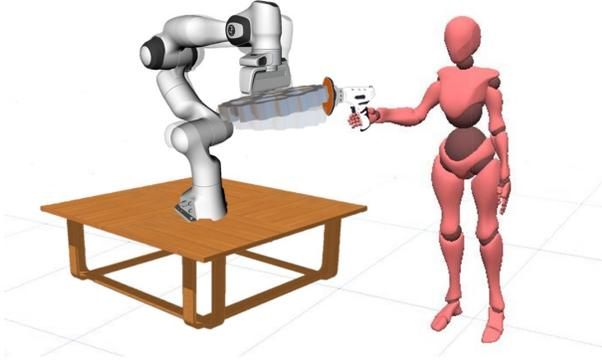
Fig. 1: Workpiece position control by the collaborative robot during a polishing process to improve the user's posture.
