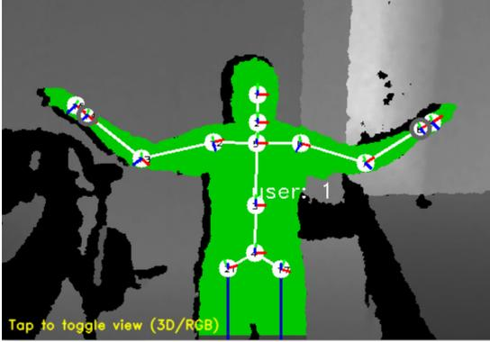
Fig. 6: Full-body skeletal tracking with the NuiTrack middleware and the Kinect v1 camera.
