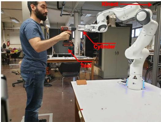
Fig. 12: The experimental setup of the collaborative polishing use case consisted of a cylinder hold by the Franka robot and polished by the user using a drilling machine equipped with a polishing wheel. A Kinect camera was placed in proximity to track the body postures.
