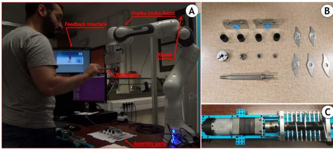
Fig. 9: The experimental setup of the collaborative assembly use case consists of the collaborative Franka robot (A). The dismantled parts of the assembly (B) are placed on the table along with the screws and the screwdrivers. The robot and the operator collaboratively assemble the crusher unit (C). A screen displays the feedback interface to the user. The skeleton tracking is achieved using a Kinect v1 camera.
