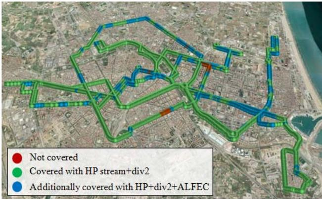
Fig. 8. Simulated coverage map of the DVB-T network in Valencia using antenna diversity, HM ( $\alpha = 1$ ) and AL-FEC (CR 3/4,  $\Delta t$  8 seconds).
