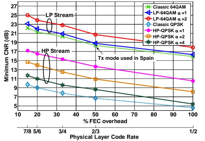
Fig. 4. Measured performance of hierarchical modulation in a Rice channel. Minimum CNR as funtion of the phisycal layer code rate.
