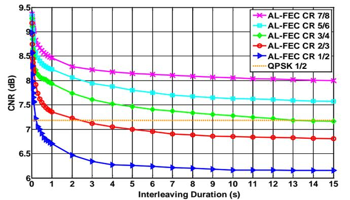
Fig. 7. Measured performance of AL-FEC in a TU6 channel with 50 Hz Doppler (115 km/h at 470 MHz, 68 km/h at 800 MHz) with HM (HP-stream, CR 2/3,  $\alpha = 1$ , FFT 8K, GI 1/4) and antenna diversity.
