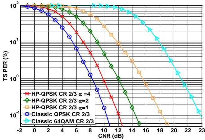
Fig. 5. Measured performance of HP stream embedded into a 64QAM hierarchical modulation in TU6 channel model (Doppler frequency 30 Hz).
