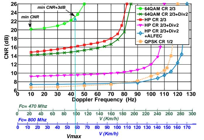
Fig. 6. DVB-T mobile performance in TU6 channel model with hierarchical modulation ( $\alpha = 1$ ), antenna diversity and AL-FEC (CR 3/4,  $\Delta t$  5 seconds). QoS criteria TS PER 1%. FFT 8K, GI 1/4.
