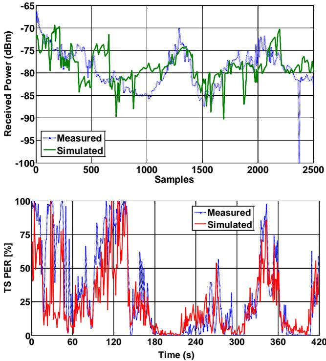
Fig. 2. Comparison between measured and simulated received power (top), and between measured and simulated TS Packet Error Rate (bottom). Route 5.
