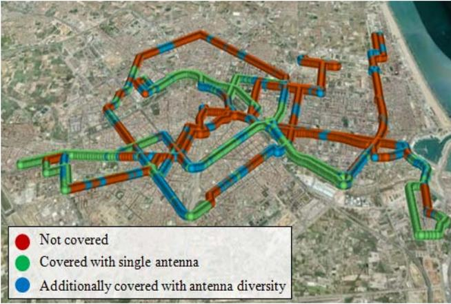
Fig. 3. Measured coverage level for single and diversity antenna reception.
