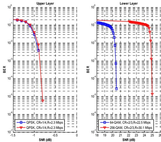
Fig. 15. Upper layer and lower layer BER performance for an RICE channel when the spectrum overlay technique is applied.
