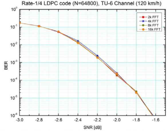
Fig. 4. Cloud Txn Layer BER for TU-6 Channel (150 Hz Doppler Rate) with Difference FFT Sizes.
