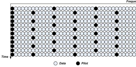
Fig. 3. Pilot pattern distribution in both time and frequency domain
