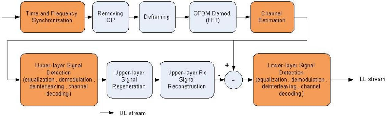
Fig. 2. Signal Detection of Multiple-Layer Cloud Txn System.
