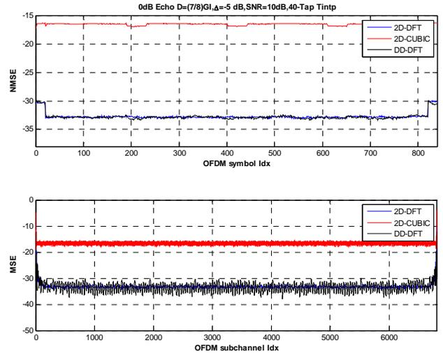
Fig. 11. Signal Cancellation Performance, 0 dB Echo ( $D=7/8$ GI), Stationary Reception, 40-tap Wiener filter,  $SNR_{LL}=10$  dB..
