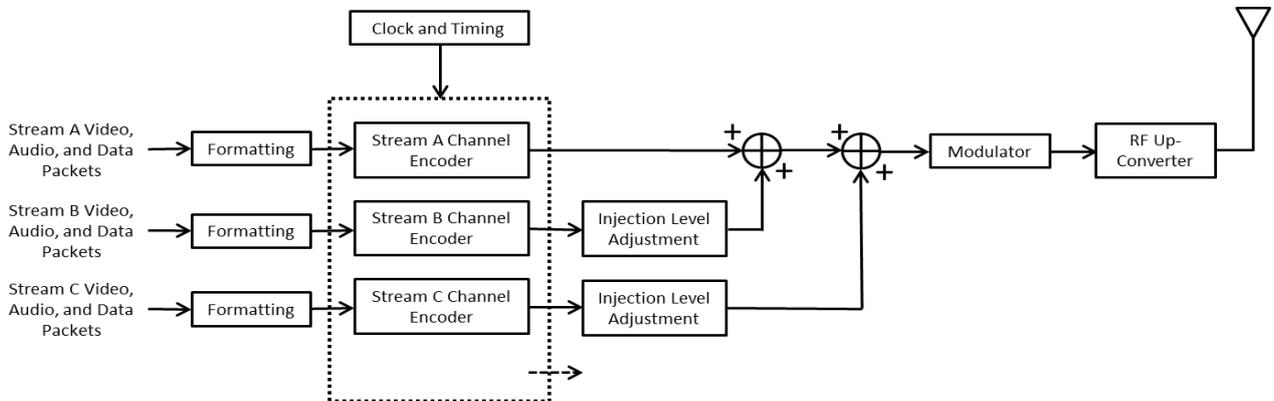
Fig. 2. Multilayer Hierarchical System transmitter.
