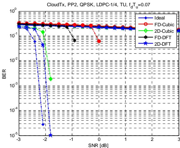
Fig. 7. Cloud Txn BER performance under a TU-6 Channel, Receiver Speed  $v = 280$  km/h
