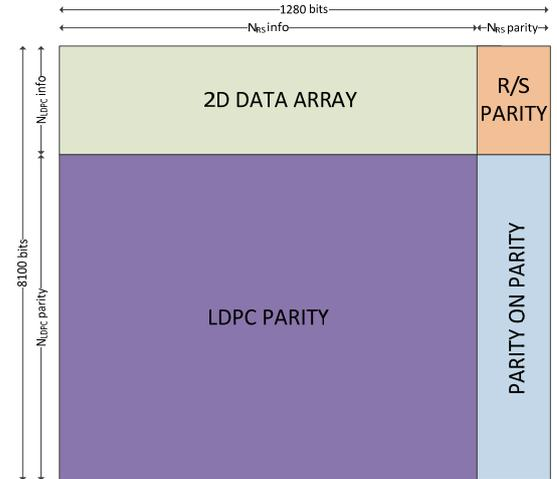
Fig. 1. A 2-Dimensional LDPC-RS code for Cloud Transmission
