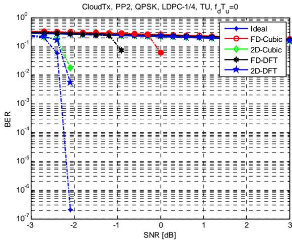
Fig. 6. Cloud Txn BER Performance under a TU-6 Channel, Stationary reception
