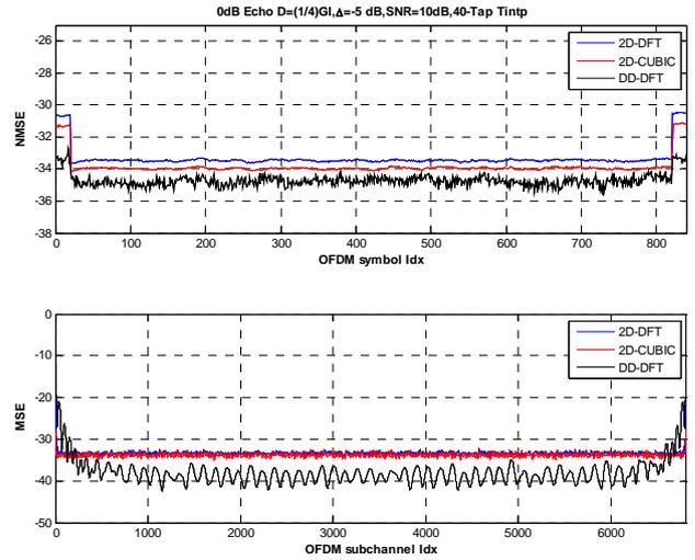
Fig. 10. Signal Cancellation Performance, 0 dB Echo ( $D=1/4$ GI), Stationary Reception, 40-tap Wiener filter,  $SNR_{LL}=10$  dB.
