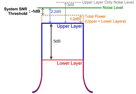
Fig. 1. Calculation of Inter-Layer Interference of a 2-Layer System
