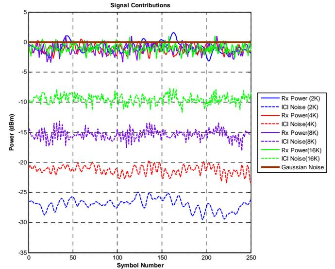
Fig. 5. OFDM Inter-Carrier Interference noise (FFT 2k, 4k, 8k and 16k, 150 Hz Doppler).
