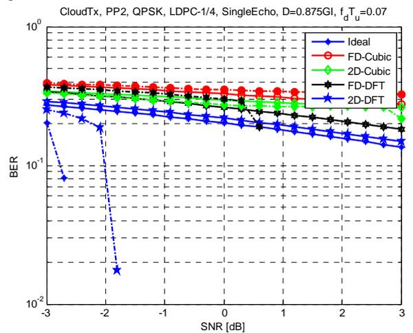
Fig. 9. Cloud Txn BER Performance, 0 dB Single Echo Channel, Receiver Speed  $v = 280$  km/h
