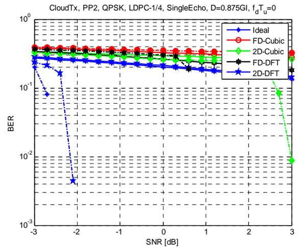
Fig. 8. Cloud Txn BER Performance, 0 dB Single Echo Channel, Stationary Reception.
