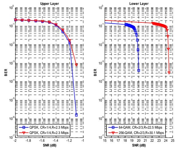
Fig. 14. Upper layer and lower layer BER performance for an AWGN channel when the spectrum overlay technique is applied.
