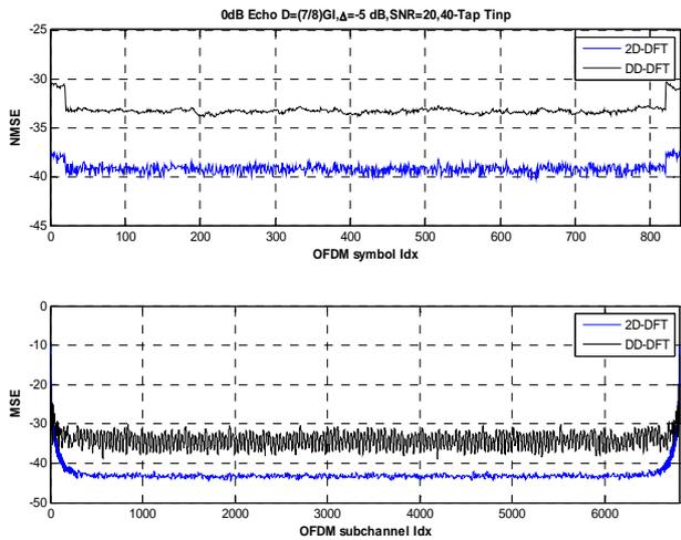
Fig. 13. Signal Cancellation Performance, 0dB Echo ( $D=7/8$ -GI), Stationary Reception, 40-tap Wiener filter,  $SNR_{LL}=20$  dB.
