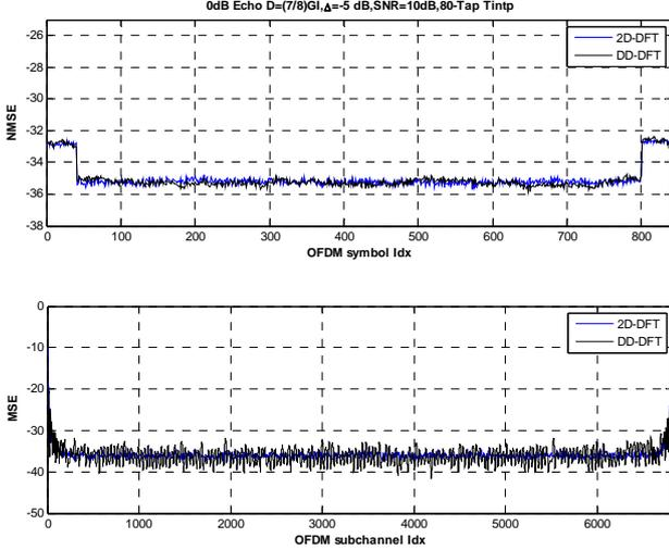
Fig. 12. Signal Cancellation Performance, 0dB Echo ( $D=7/8$ -GI), Stationary Reception, 80-tap Wiener filter,  $SNR_{LL}=10$  dB.
