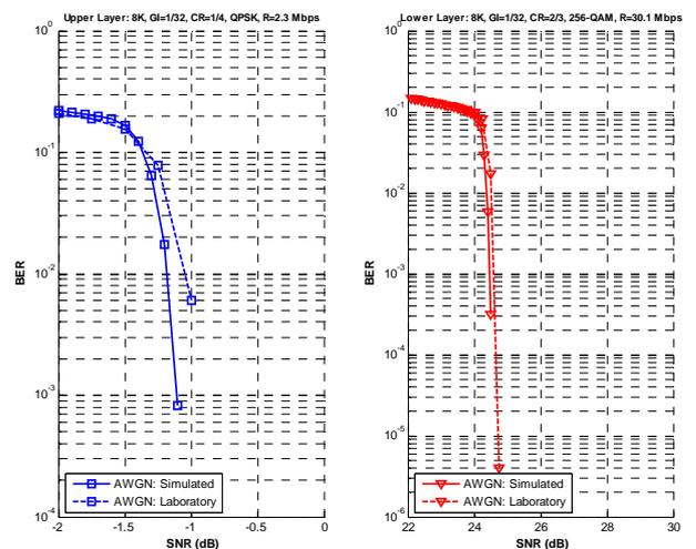
Fig. 17. Laboratory BER Curves for a two layer system (Upper layer Cloud Txn, Lower Layer DVB-T2, Injection rate 5 dB).
