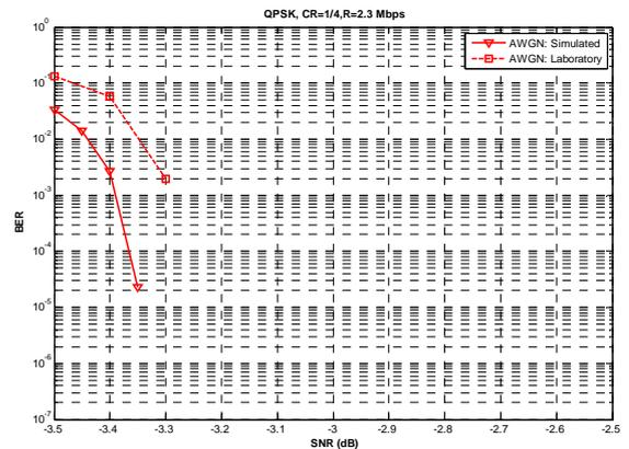
Fig. 16. Simulated vs laboratory BER Curves for a single layer system
