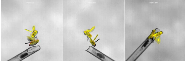
Fig. 5. Performance of the fly tracking algorithm on the three camera views for a particular image frame. Tracking results from previous few frames are superimposed for clarity.
