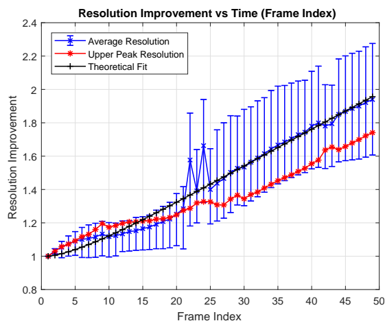
Fig. 16. Resolution improvement vs time of GTT traces (Section IV-B).
