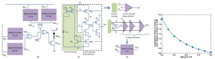
Fig. 13. Illustration of the initialization circuit. (a) Circuit connections of the initialization circuit. (b) Current sensing circuit to current starved delay element connection. (c) Symbolic representation of the circuit in (b). (d) Illustration of each pixel's Sense to Pulse circuit. (e) Propagation delay of  $Out_{i,j}$  with respect to  $En_{H,V}$  vs. Ip(i,j).
