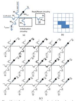
Fig. 10. (a) Implementation of each pixel for voltage based memristive devices. (b) A sample pattern of ant traversal. (c) Illustration of connections of adjacent pixels for voltage based memristive devices.
