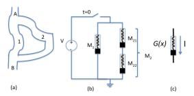
Fig. 1. (a) Points A (nest) and point B (food source) are connected through two paths L1 and L2, such that L2=2L1. (b) Memristive network model of the ant colony model in (a).
