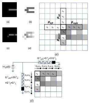
Fig. 8. Illustration of memristive implementation of ant colony algorithm for a small image. (a,b) original image and its edges. (c,d) noisy image and its edges. (e) probability of ant traversal for all of the paths in the path set. (f) Memristive implementation of (e).
