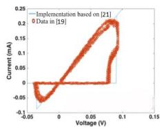
Fig. 12. Comparison of the implementation of model in [21] with the experimental data in [19].
