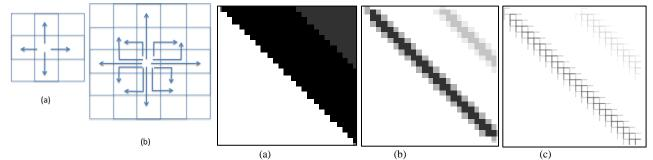
Fig. 2. (a) Path set illustration for L=1. (b) Path set illustration for L=2.
