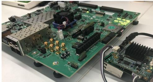
Figure 7: ZU9(left) and ZU2(right) FPGA Devices
