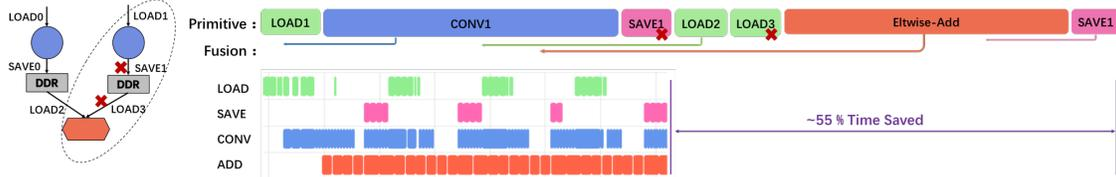
Figure 9: Optimized pipeline achieved by fusing one of convolutions and the adjacent eltwise-add by DNNVM.
