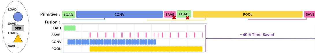
Figure 8: Optimized pipeline achieved by fusing the adjacent convolution and pooling by DNNVM.
