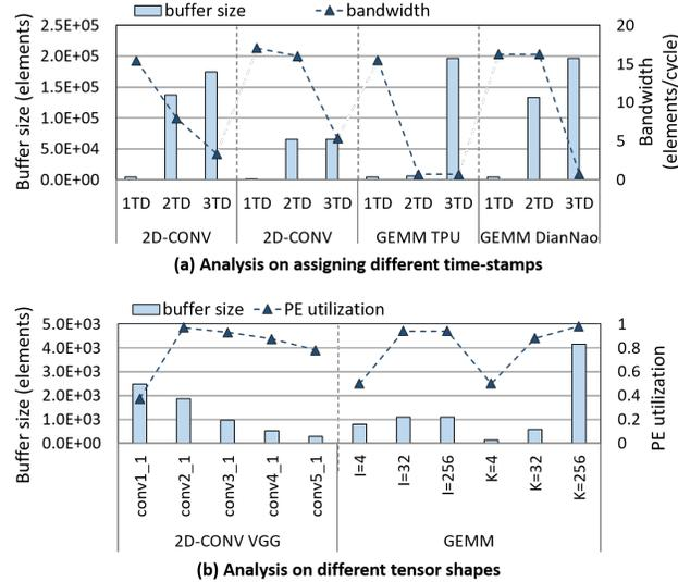
Fig. 9. Analyzing the trade-off between buffer size, bandwidth, PE utilization using data layout IR.
