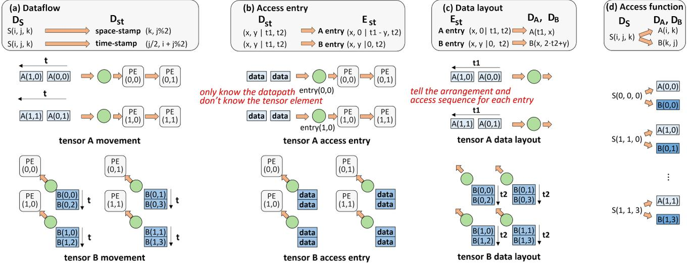
Fig. 3. GEMM dataflow decomposition example. The dataflow is decomposed into access entry IR and data layout IR.
