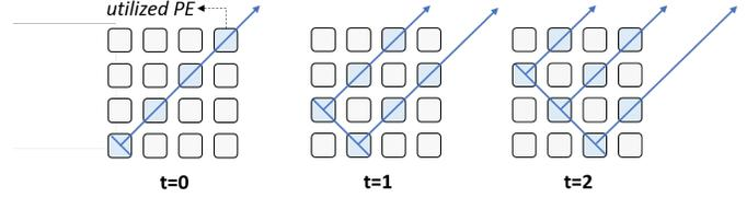
Fig. 11. TENET inferior dataflow with under-utilized PE.
