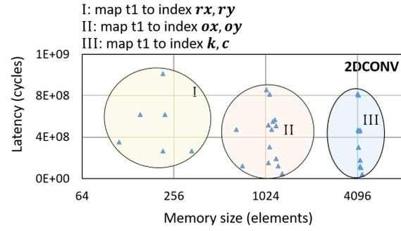
Fig. 8. Using Rubick data layout IRs to explore hardware design.  $rx, ry, ox, oy, k, c$  are tensor indices in Equation 10
