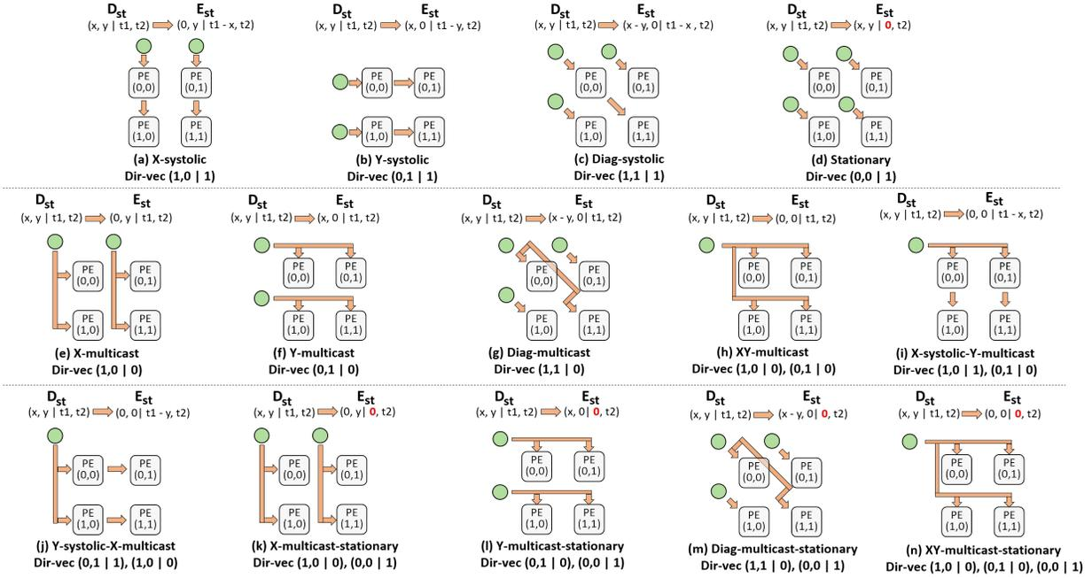
Fig. 4. Input access entry space on 2D-PE array. The space is formulated as tensor access direction vectors.
