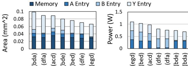
Fig. 13. Area and power breakdown via GEMM dataflow decomposition. The X-axis is different dataflows notated by access entry. E.g., (bda) means, tensor A, B, Y applies type-(a), type-(d), type-(b) access entry of Figure 4.
