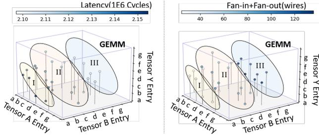
Fig. 7. Using Rubick access entry IRs to explore hardware design. a-g means the access entry type in Figure 4.
