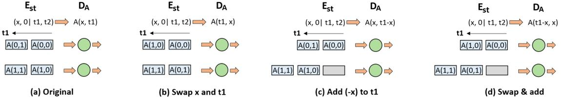
Fig. 5. Data layout space on 2D-PE array. The space is formulated as linear matrix transformation.
