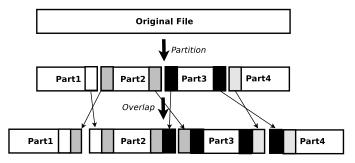
Fig. 3. Chunk overlap to reduce overhead in relays.
