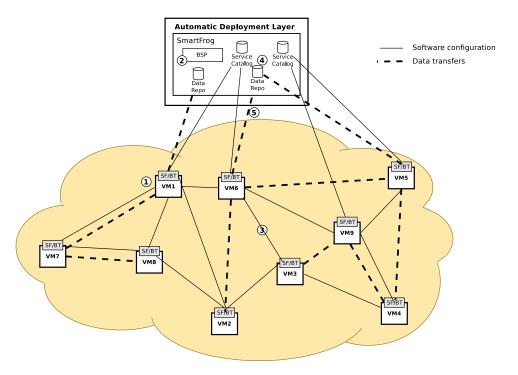
Fig. 4. P2P interactions between our SF/modified BitTorrent daemons and the Automatic Deployment Layer.
