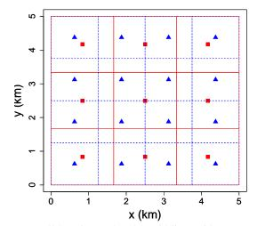
(a) Non-collaborative mode. The solid lines grid represents the Voronoi cells for Op1 (red squares) while the dotted lines grid represents the Voronoi cells for Op2 (blue triangles).
