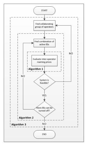
Fig. 1: Top level activity diagram of the proposed virtualization framework.
