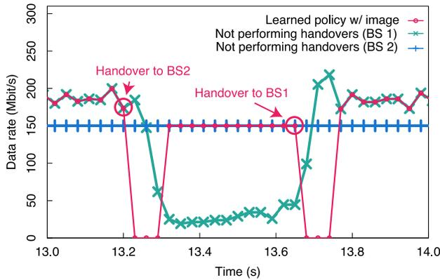
(a) Portion of the time series of the data rate and handover timing learned when the camera monitors with angle A.
