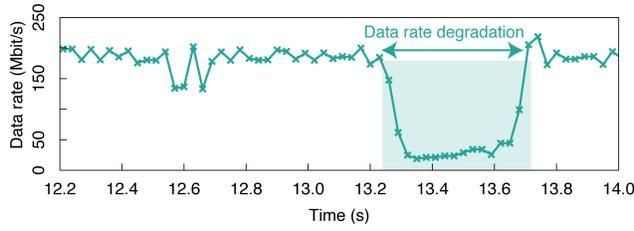
(a) Time series of the data rate provided by BS 1 obtained when the camera monitors with angle A.
