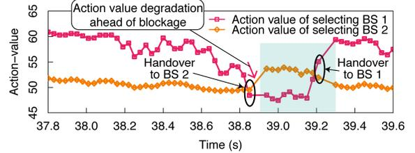
(d) Time series of action value in proposed framework when the camera monitors with angle B.
