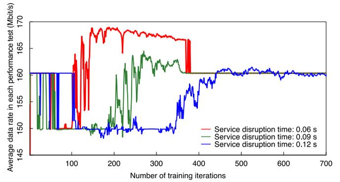
Fig. 13. Average data rate in each performance test corresponding to a training iteration.
