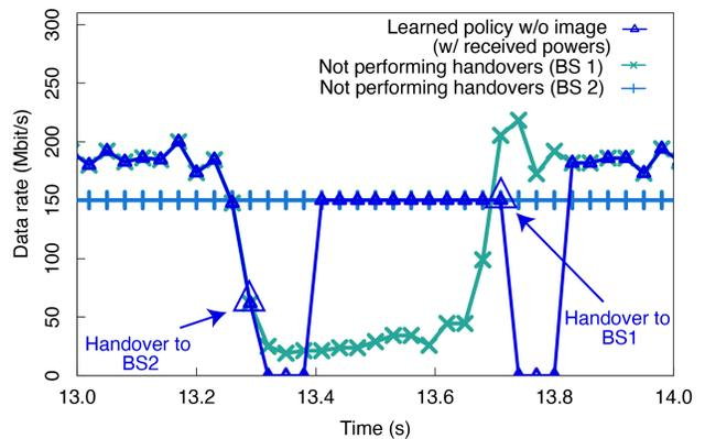
Fig. 5. Example of handover timing when  $T_{\text{dis}} = 0.09$  s. Handovers are performed after the variation in the data rate provided by BS 1.
