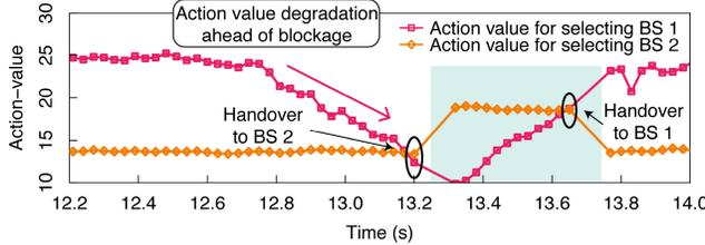
(c) Time series of action value in proposed framework when the camera monitors with angle A.
