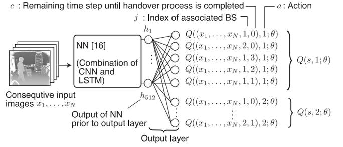
Fig. 6. NN architecture for approximating optimal action-value function  $Q^*(s, a)$  defined in (2) for  $\mathcal{C} = \{0, 1, 2, 3\}$  and  $\mathcal{J} = \{1, 2\}$ . With the exception of the output layer, the architecture herein is identical to that used in [37]. The architecture is a combination of a CNN, which deals with images, and an LSTM, which deals with sequential inputs [45].
