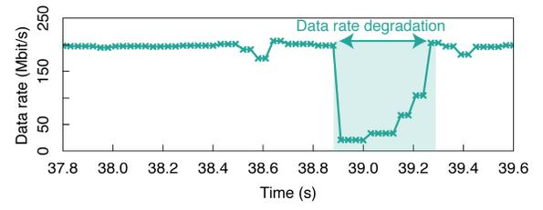
(b) Time series of the data rate provided by BS 1 obtained when the camera monitors with angle B.
