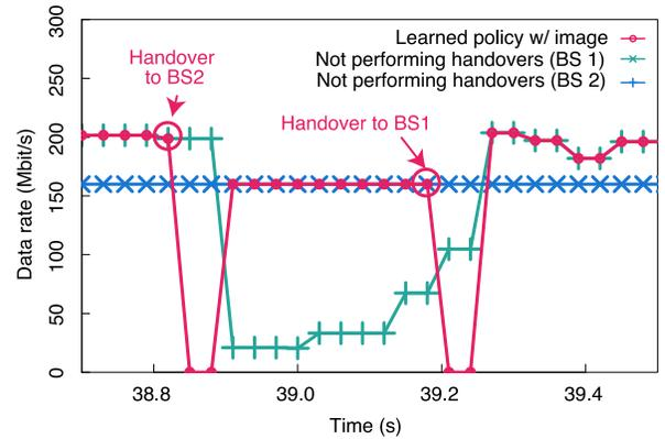
(b) Portion of the time series of the data rate and handover timing learned when the camera monitors with angle B.
