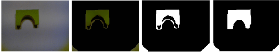
Figure 5: Image processing - original image, removal of the background, converting to BW image and filling the holes
