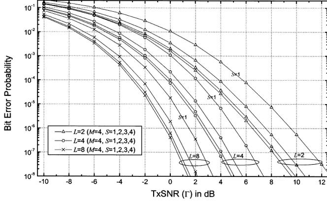
Fig. 4. Average BEP performance for various  $L$  as a function of TxSNR  $\Gamma$ , when  $M = 4$ .
