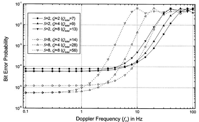
Fig. 6. Average BEP performance as a function of Doppler frequency  $f_D$ , when  $M = 8$ ,  $L = 1$ ,  $\Gamma = 5$  dB, and  $f_b = 1500$  b/s.
