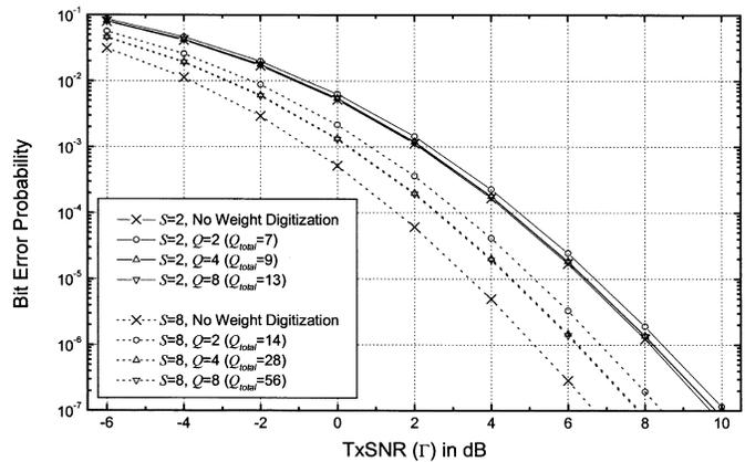
Fig. 5. Average BEP performance for various  $Q$  as a function of TxSNR  $\Gamma$ , when  $M = 8$  and  $L = 1$ .
