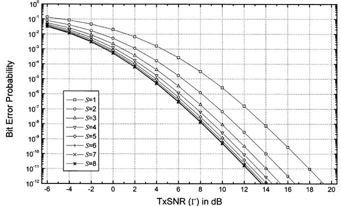
Fig. 2. Average BEP performance for various  $S$  as a function of TxSNR  $\Gamma$ , when  $M = 8$  and  $L = 1$ .
