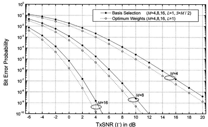
Fig. 3. Average BEP performance for various  $M$  as a function of TxSNR  $\Gamma$ , when  $L = 1$  and  $S = M/2$ .
