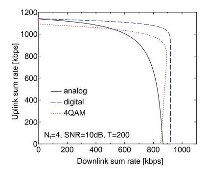
Fig. 4. Downlink vs. uplink tradeoff for  $N_t = 4$ ,  $\rho = 10$  dB, T = 200 symbols.
