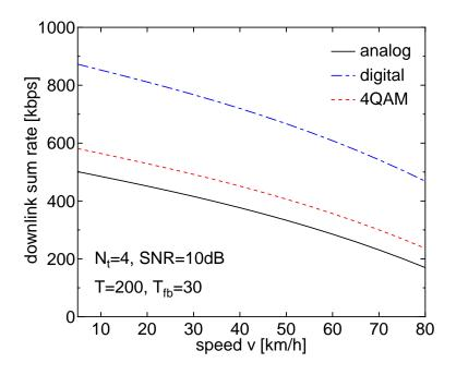
Fig. 8. Downlink rate vs. mobile speed for  $T_{\rm fb} = 30$ , T = 200.
