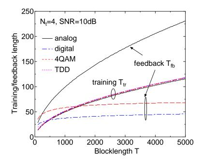
Fig. 2. Feedback/training length vs. block length for  $N_t = 4, \rho = 10$  dB.
