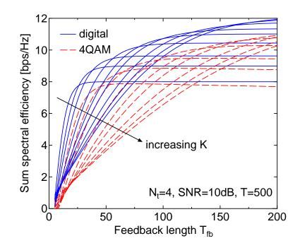
Fig. 10. Downlink sum spectral efficiency vs. feedback symbols ( $T_{\rm fb}$ ) for T = 500,  $N_t = 4$ ,  $\rho = 10$  dB, for K from 4 to 31 users.
