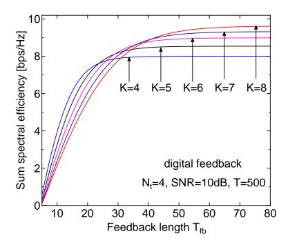
Fig. 9. Downlink sum spectral efficiency vs. feedback symbols ( $T_{\rm fb}$ ) for T = 500,  $N_t = 4$ ,  $\rho = 10$  dB, for K from 4 to 8 users.
