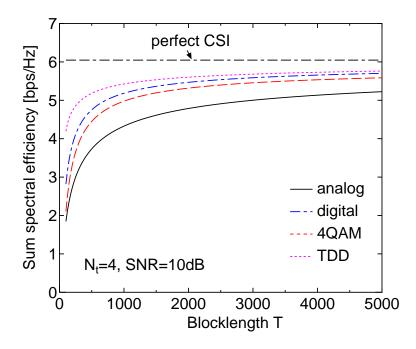
Fig. 3. Sum spectral efficiency vs. block length T.
