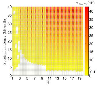
Fig. 4. Approximation error in terms of  $E_b/N_0$  (dB) between the nearlyexact  $E_b/N_0$  and the approximation method of [6] as a function of the SE and  $\overline{\beta} = \max\{t, r\}/\min\{t, r\}$ .
