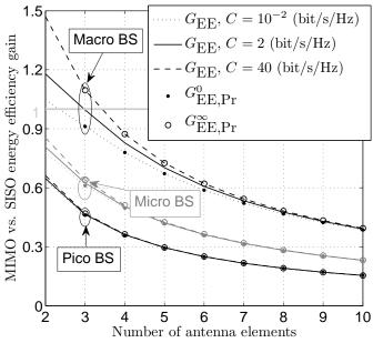
Fig. 9. MIMO vs. SISO EE gain against the number of antennas  $n_{ant} = t = r$  for different types of BS when considering the double linear PCM of (6).
