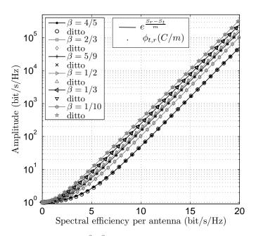
Fig. 2. Comparison of  $e^{\frac{S_r-S_t}{m}}$  with our parametric function  $\phi_{t,r}(C/m)$  as a function of the SE per antenna for various receive/transmit antenna ratios.
