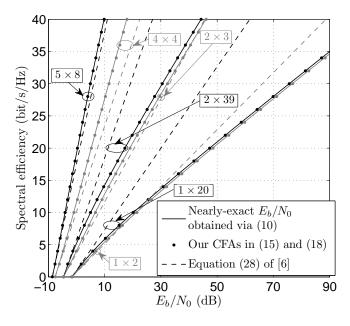
Fig. 5. Comparison of our EE-SE trade-off CFAs in (15) and (18) with the approximation method of [6] and the nearly-exact  $E_b/N_0$  obtained via (10) for various  $r \times t$  antenna configurations.
