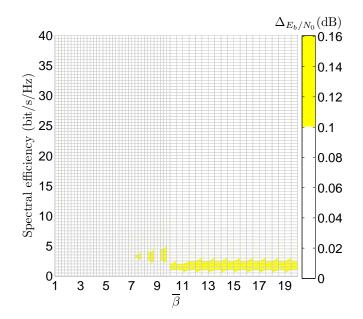
Fig. 3. Approximation error in terms of  $E_b/N_0$  (dB) between the nearlyexact  $E_b/N_0$  and our CFAs in (15) and (18) as a function of the SE and  $\overline{\beta} = \max\{t, r\}/\min\{t, r\}$ .
