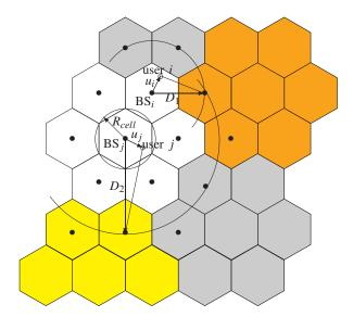
Fig. 2. System layout with clusters of seven cells of radius  $R_{cell}$  (the radius of the circle circumscribing the cell) with an example of two users, with the distances  $D_1$  and  $D_2$ , respectively, from their BS to the interfering BSs.
