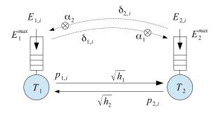
Fig. 1. Two-way channel with energy harvesting transmitters and energy cooperation.
