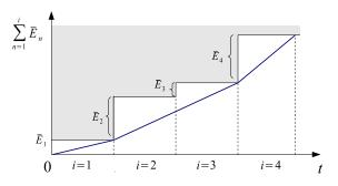
Fig. 6. Optimal sum-power policy for an energy cooperating MAC for a deadline of N = 4 time slots.
