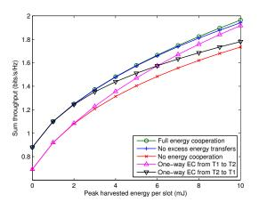
Fig. 9. Sum-throughput for the two-way channel with one-way energy transfer, and without excess energy transfers  $\epsilon_{k,i}$ .
