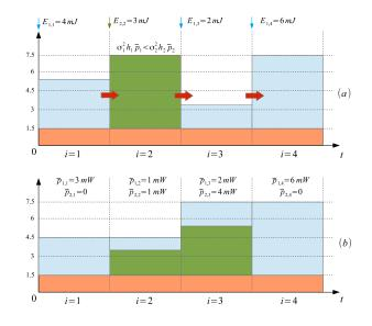
Fig. 4. Directional water-filling (a) initial levels and (b) levels after water flow, for an example setting with N = 4. The blue, green and orange areas correspond to source consumption  $\bar{p}_1$ , relay consumption  $\bar{p}_2$  and the constant term in (25), respectively.
