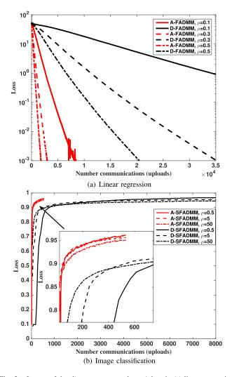
Fig. 5. Impact of the *disagreement penalty weight*  $\rho$  in (a) linear regression and (b) image classification using DNNs.
