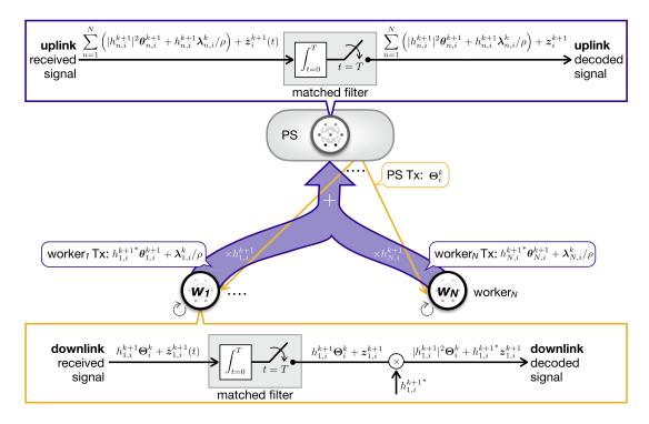
Fig. 2. An illustration of uplink and downlink communication in A-FADMM under channel noise.
