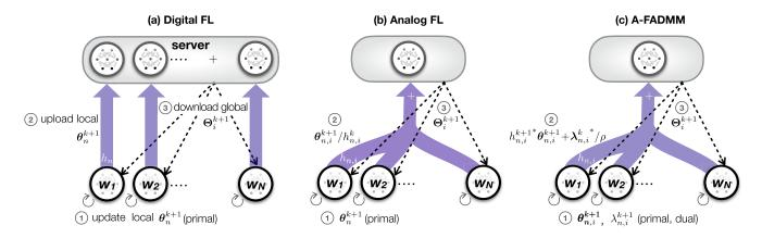
Fig. 1. Schematic illustrations of: (a) digital federated learning (FL), (b) analog FL with channel inversion, and (c) analog-federated ADMM (A-FADMM) without channel inversion.
