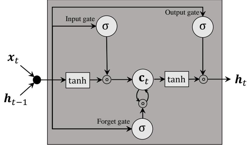
Fig. 2. Structure of the basic LSTM model
