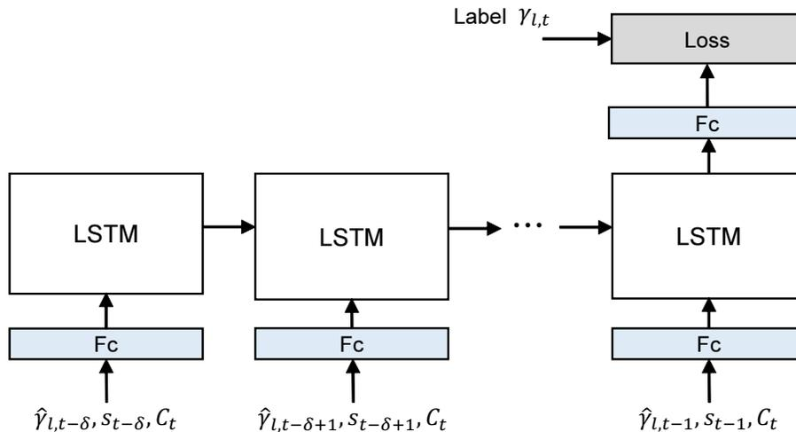
Fig. 4. Structure of the LSTM-based prediction model
