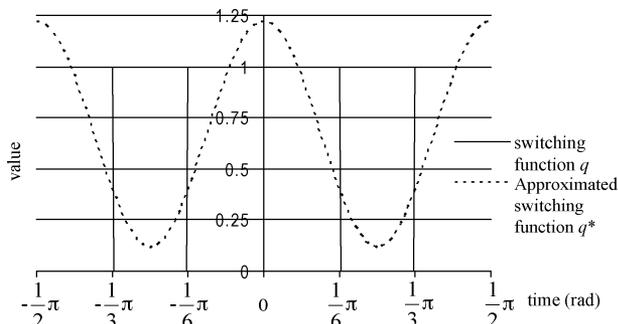
Fig. 6. Example of switching function and approximated switching function in Mathieu's equation ( $\beta = (2/3)\pi$ ).
