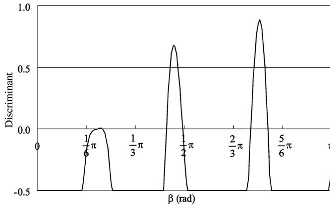
Fig. 7. Variation of discriminant for characteristic equation of Hill's equation to parameter  $\beta$ .
