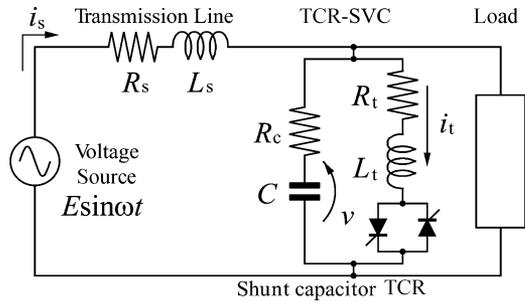
Fig. 1. Schematic diagram of single phase TCR-SVC.
