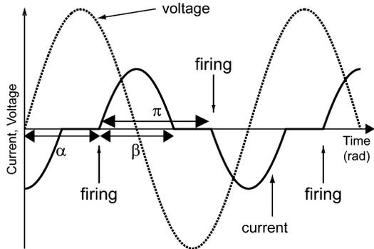
Fig. 2. Ideal voltage and current waveforms of TCR.
