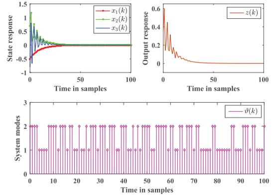
Fig. 6. The state and output responses of the closed-loop system and the evolution of system mode  $\vartheta(k)$ .
