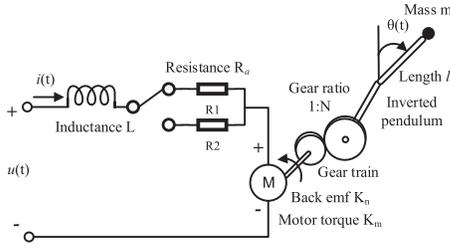
Fig. 5. Structure of inverted pendulum controlled by DC motor.
