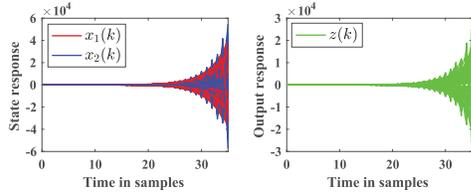
Fig. 2. The state and output responses of the open-loop system over 100 realizations.
