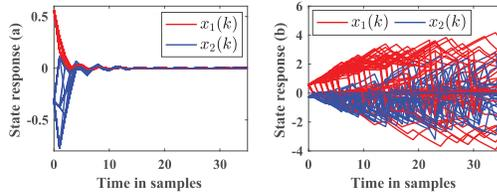
Fig. 4. The state responses of the closed-loop SMJSPS with (a)  $l_1 = 0.75$ ,  $l_2 = 0.82$ ,  $l_3 = 0.88$ ,  $h_1 = 0.92$ ,  $h_2 = 0.95$ ,  $h_3 = 0.98$  and (b)  $l_1 = 16$ ,  $l_2 = 15$ ,  $l_3 = 17$ ,  $h_1 = 14$ ,  $h_2 = 17$ ,  $h_3 = 16$  over 100 realizations.
