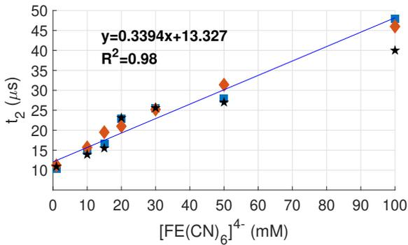
Fig. 10. Measurements of different  $t_2$  for different concentrations of  $[\text{Fe}(\text{CN})_6]^{4-}$  diluted in PBS 1X solution.
