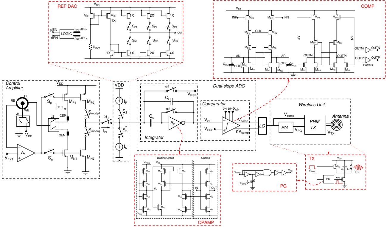
Fig. 3. Detailed schematic of a potentiostat channel. The polarity of the potentiostat is selected manually via J1, J2 and static switches  $S_n$  and  $S_p$ .
