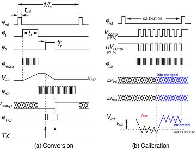
Fig. 4. Detailed timing diagram of the operation of the potentiostat channel in (a) conversion and (b) calibration mode.
