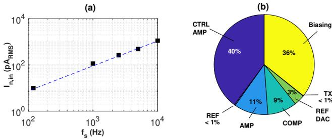
Fig. 7. (a) RMS input current noise for different sampling frequencies and (b) potentiostat channel power breakdown estimated at a sampling frequency of 1 kHz and equal to 12  $\mu$ W from a 1.2V supply.
