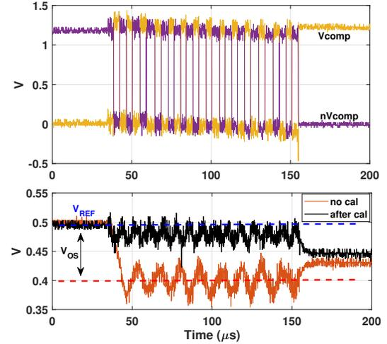
Fig. 8. Calibration of ADC offset.
