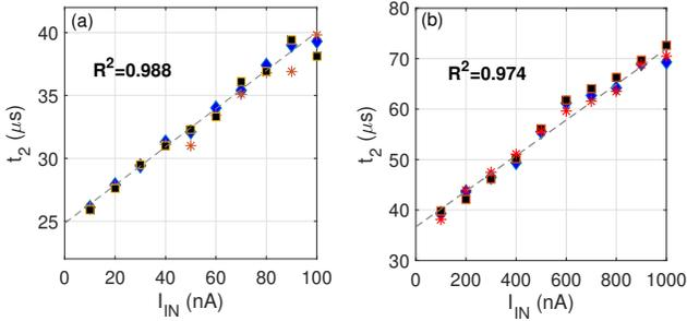
Fig. 6. Linearity of the ADC for a input current range between (a) 10nA and 100nA and (b) 100nA to 1 $\mu$ A.
