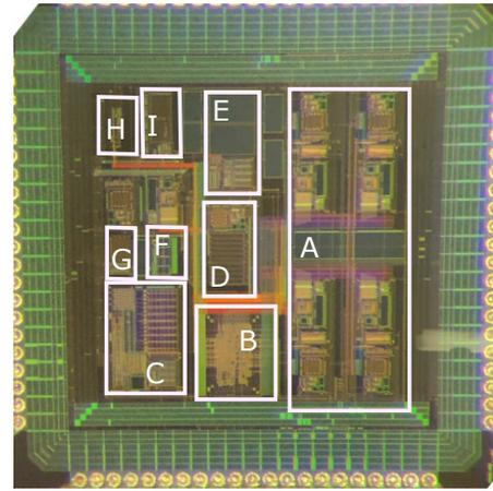
Fig. 5. Chip Layout. **A.** 4-channel dual-slope ADC with control amplifier; **B.** 8-register SPI; **C.** Bandgap; **D.** 1.2V voltage regulator; **E.** Bias cell; **F.** Power-on reset; **G.** Beta multiplier; **H.** TX; Unlabeled blocks represent test structures.
