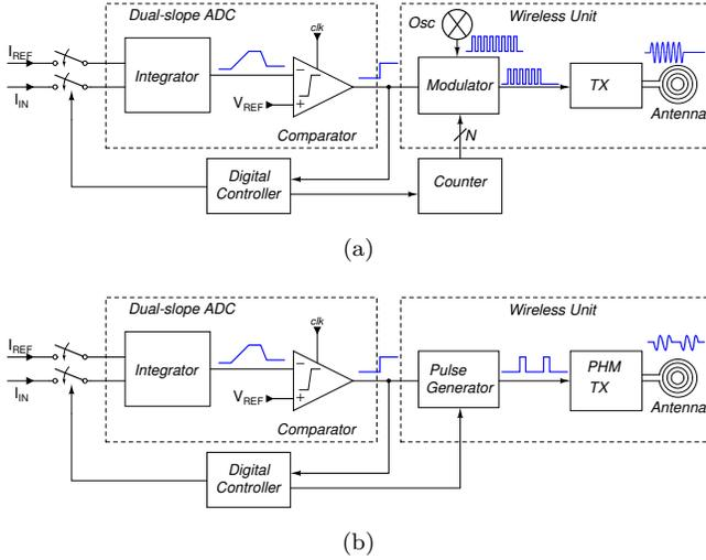
Fig. 1. Wireless potentiostat architecture. (a) Conventional and (b) proposed system.
