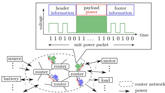
Fig. 1: Concept of power packet and its dispatching system.
