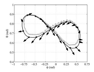
Figure 14: Filtered position in the  $(\phi, \theta)$  plane obtained with the third approach without the IMU (solid line and ' $\circ$ ') and related velocity angle estimates (arrows). The raw position data is shown with gray '\*'. Design parameters:  $\lambda = 500$ ,  $K_{\gamma} = [0.4, 0.9]^T$ . Wing size: 12 m<sup>2</sup>, wind speed: 2.3 m/s at 4 m from the ground.
