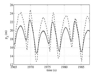
Figure 10: Experimental results. Estimates of the position along the Z axis,  $p_Z(t)$ , obtained with either the first and second (dashed line) or the third (solid) approach.
