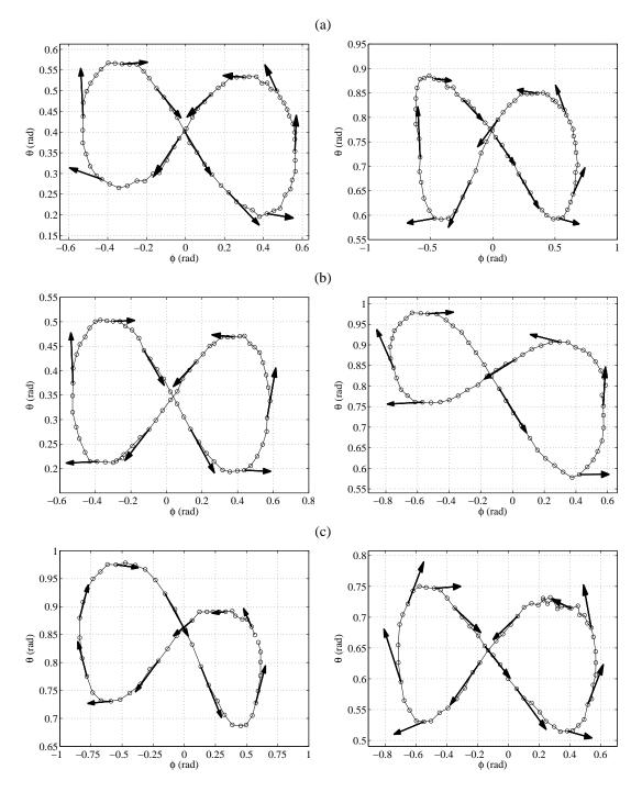
Figure 15: Experimental results. Examples of wing paths (solid lines with ' $\circ$ ') and velocity angles (arrows) obtained with a (a) 6 m<sup>2</sup>, (b) 9 m<sup>2</sup> and (c) 12 m<sup>2</sup> wing and with about 2 m/s (left) and 4 m/s (right) wind speed measured at 4 m above the ground.
