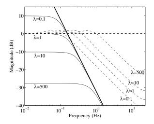
Figure 7: Bode plot of the magnitude of the discrete-time transfer functions  $F_u^{\text{KF}}(z) \doteq \hat{p}_X(z)/\hat{p}_X(z)$  (solid lines) and  $F_y^{\text{KF}} \doteq \hat{p}_X(z)/\hat{p}_X(z)$  (dashed lines) for different values of weighting ratio  $\lambda \doteq Q/R$ , together with their respective asymptotic behaviors (thick lines).
