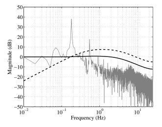
Figure 8: Bode plot of the magnitude of the discrete-time transfer functions  $F_{y_1}^{\text{LO}}(z) \doteq \hat{\gamma}(z)/\tilde{\gamma}(z)$  (solid lines) and  $F_{y_2}^{\text{LO}}(z) \doteq \hat{\gamma}(z)/\tilde{\gamma}(z)$  (dashed lines) obtained with the observer's gain  $K_{\gamma} = [0.4 \ 0.9]^T$ , and magnitude of the fast Fourier transform of the input signal  $\tilde{\gamma}(z)$  (gray line).
