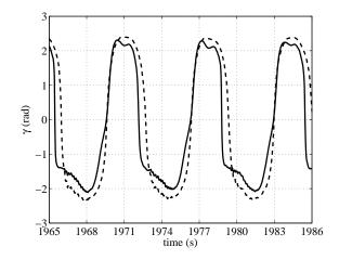
Figure 12: Time courses of the filtered velocity angle  $\hat{\gamma}$  obtained in the third approach with the IMU (solid line) and without (dashed line). Design parameters:  $\lambda = 500$ ,  $K_{\gamma} = [0.4, 0.9]^T$ . Wing size: 12 m<sup>2</sup>, wind speed: 2.3 m/s at 4 m from the ground.
