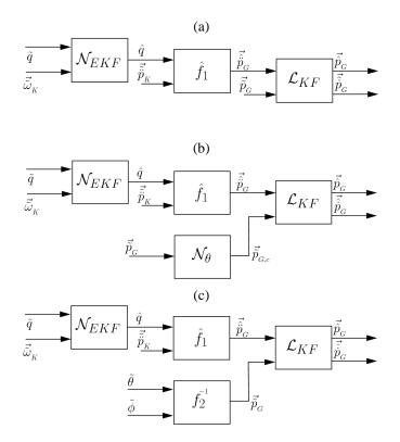
Figure 6: Schemes of the designed observers for the first, second and third approach ((a), (b) and (c), respectively).
