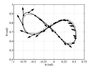
Figure 13: Filtered position in the  $(\phi, \theta)$  plane obtained with the third approach with the IMU (solid line and 'o') and related velocity angle estimates (arrows). The raw position data is shown with gray '\*'. Design parameters:  $\lambda = 500$ ,  $K_{\gamma} = [0.4, 0.9]^T$ . Wing size: 12 m<sup>2</sup>, wind speed: 2.3 m/s at 4 m from the ground.
