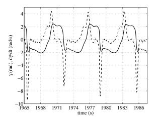
Figure 11: Time courses of the filtered velocity angle  $\hat{\gamma}$  (solid line), and its derivative  $\hat{\dot{\gamma}}$  (dashed line). Design parameters:  $\lambda = 500, K_{\gamma} = [0.4, 0.9]^T$ . Wing size: 12 m<sup>2</sup>, wind speed: 2.3 m/s at 4 m from the ground.
