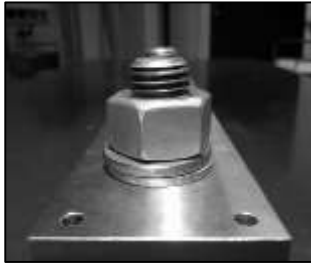
Fig. 12. The ‘two washers’ error scenario. The 2 nd washer will cause an error detection within stage 3 or 4 , since the desired angular position of the nut will not be reached.
