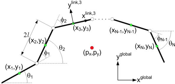
Fig. 1. Kinematic parameters of the snake robot.
