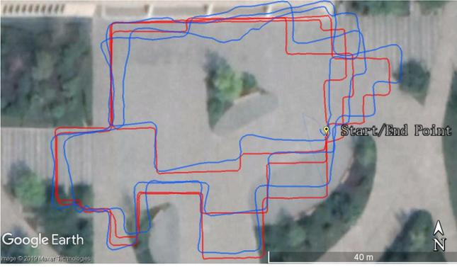
Fig. 20. Outdoor walking trajectory beside tall buildings overlaid with Google Earth (blue line: Samsung S10 GPS positioning; red line: ZUPT + RNG PNS positioning result).
