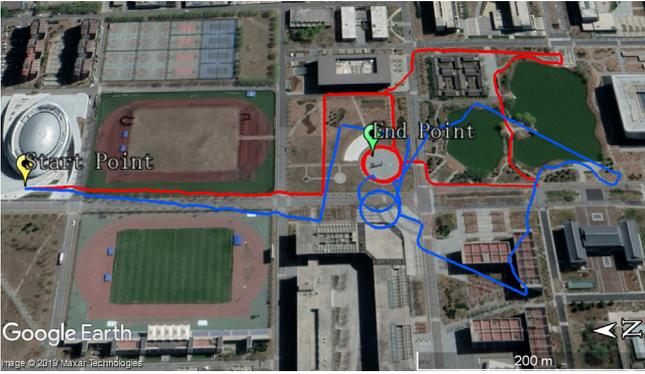
Fig. 21. Estimated trajectory of longer outdoor walking (blue line: ZUPT positioning result for left foot; red line: ZUPT + RNG positioning result)
