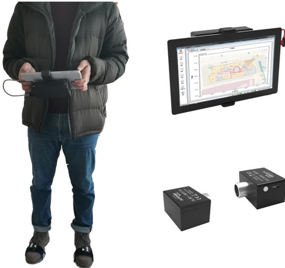
Fig. 16. Left: System overview. Upper right: data processing/display module. Low right: IMU and ultrasonic ranging modules
