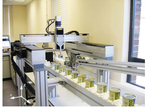
Fig. 2: The gantry robot.
