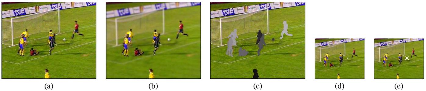
Fig. 3. Examples of encoding modalities. (a) Sample frame from the sequence *Soccer*; (b) Semantic frame-based encoding: the background is selectively lowpass-filtered prior to encoding; (c) Metadata-based encoding: object shapes are superimposed on the background; (d) Spatial resolution reduction; (e) Metadata-enhanced encoding: metadata are used to enhance relevant portions of a video
