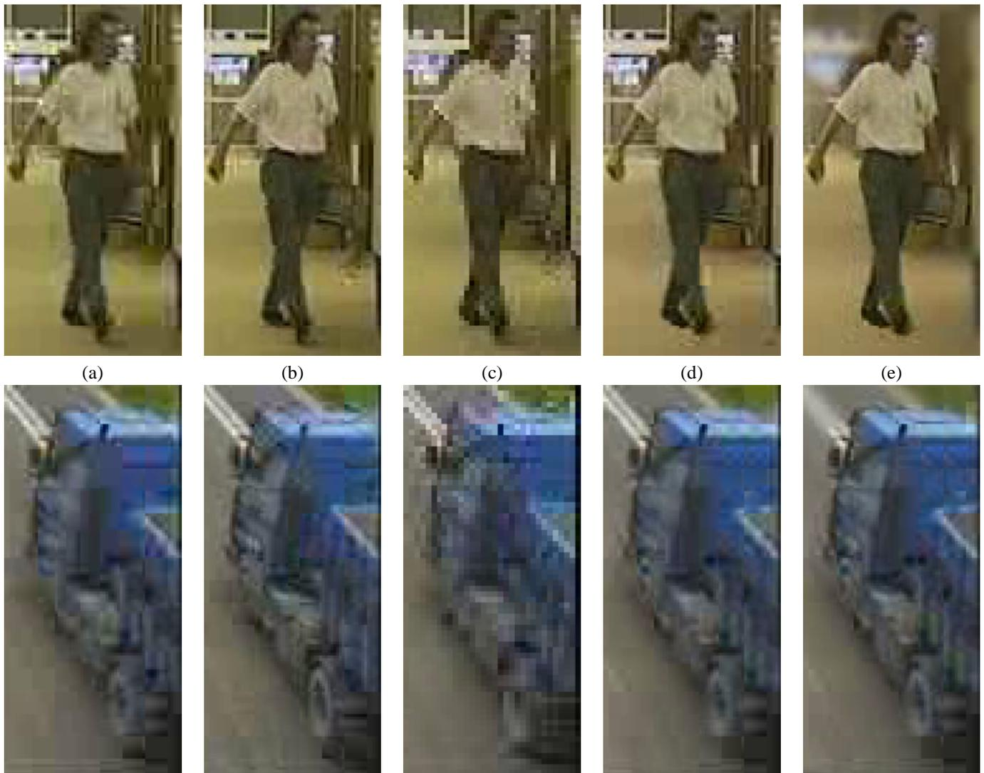
Fig. 8. Details of frame 280 of *Hall monitor* (top) and frame 16 of *Highway* (bottom). The sequences are encoded with MPEG-1 at 150 Kbit/s using different encoding modalities: (a) coded original sequence; (b) temporal resolution reduction; (c) spatial resolution reduction; (d) static background; (e) simplified background
