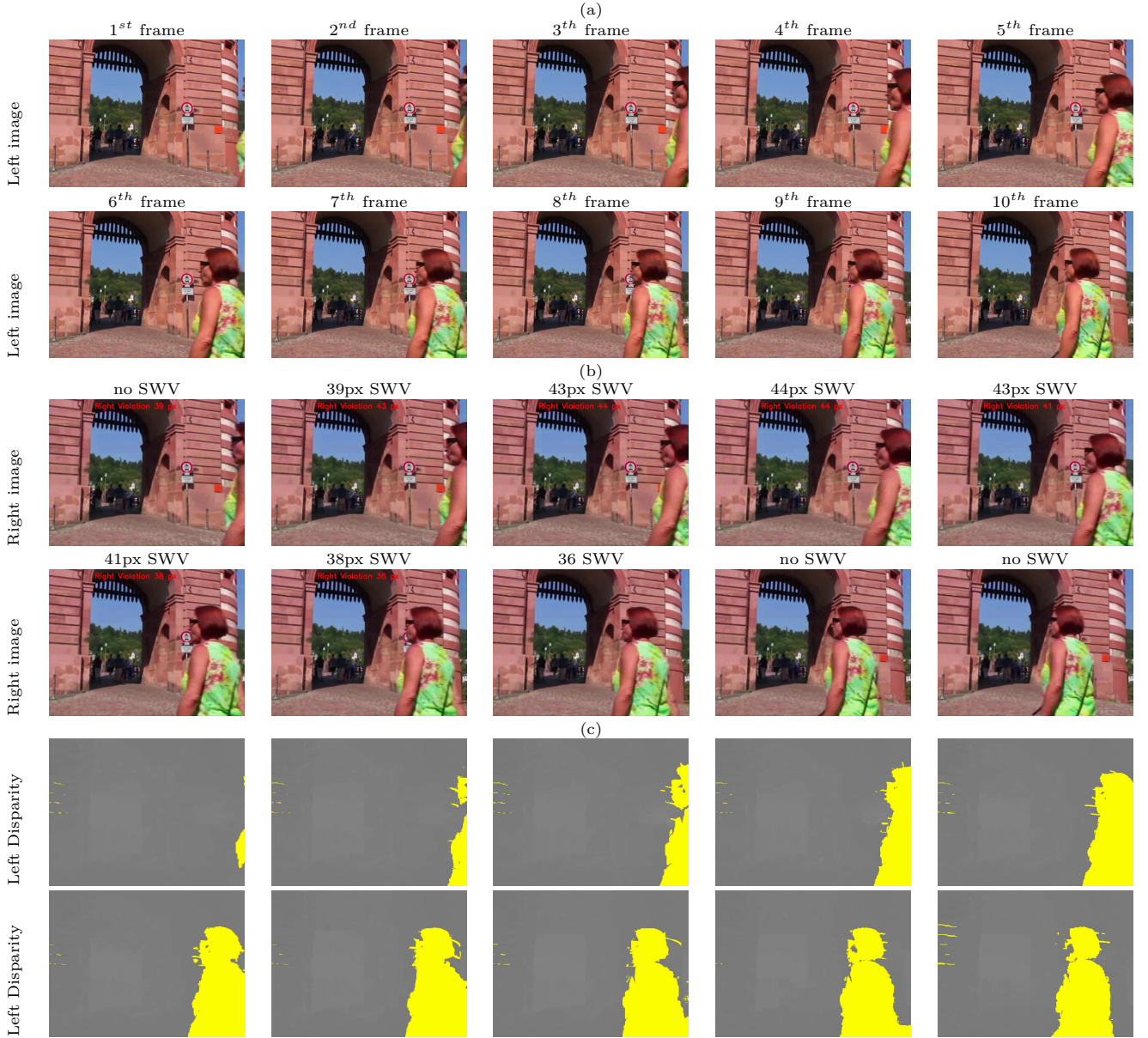
Fig. 4. Example of right stereoscopic violation: a) left video frames, and corresponding b) right video frames, c) left disparity maps.
