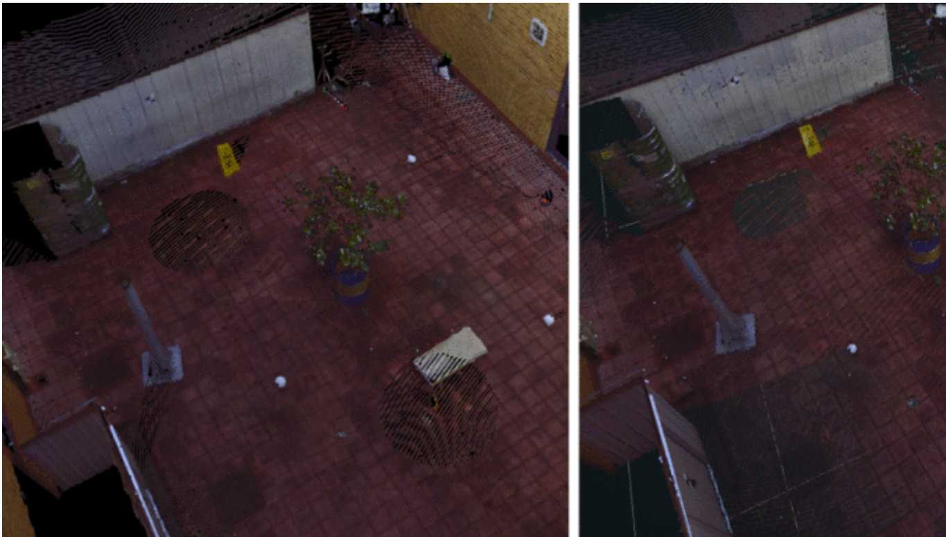
Rendering of our method (left) and [31] (right). The latter features white artifacts between the cells used for the data structure.
