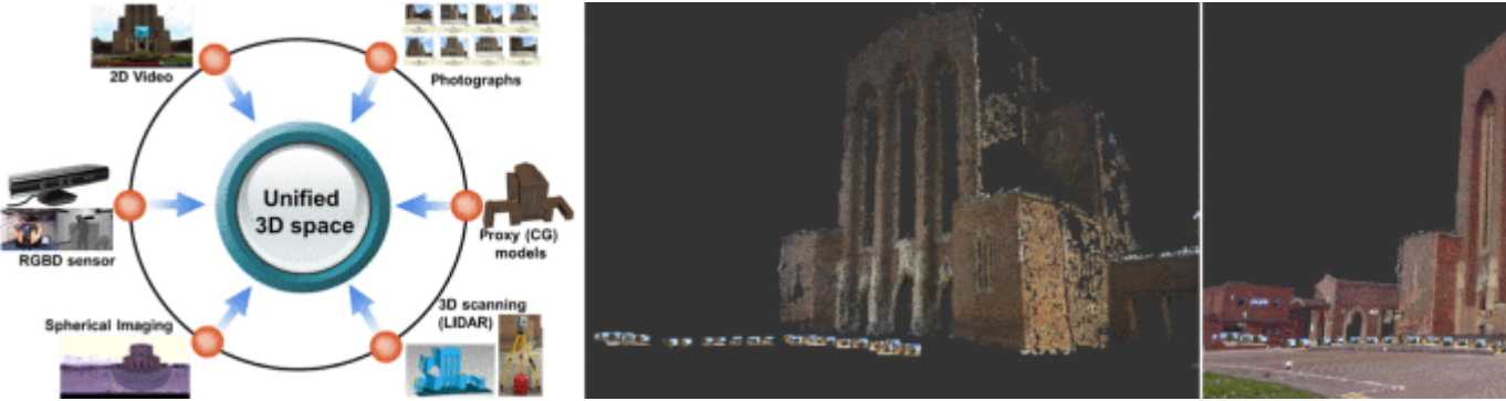
Multimodal data registration and visualization. Left: overview of multimodal visual data registration. Middle: multiple photographs and their 3D reconstruction. Right: registration to LIDAR coordinate system.
