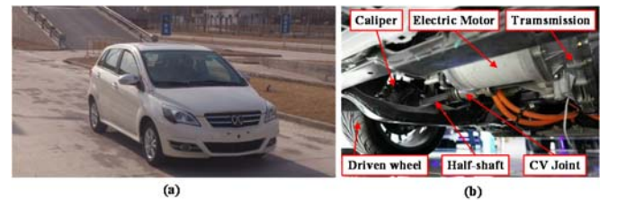
Fig. 3. Pictures of the test vehicle and the electrified powertrain system.
