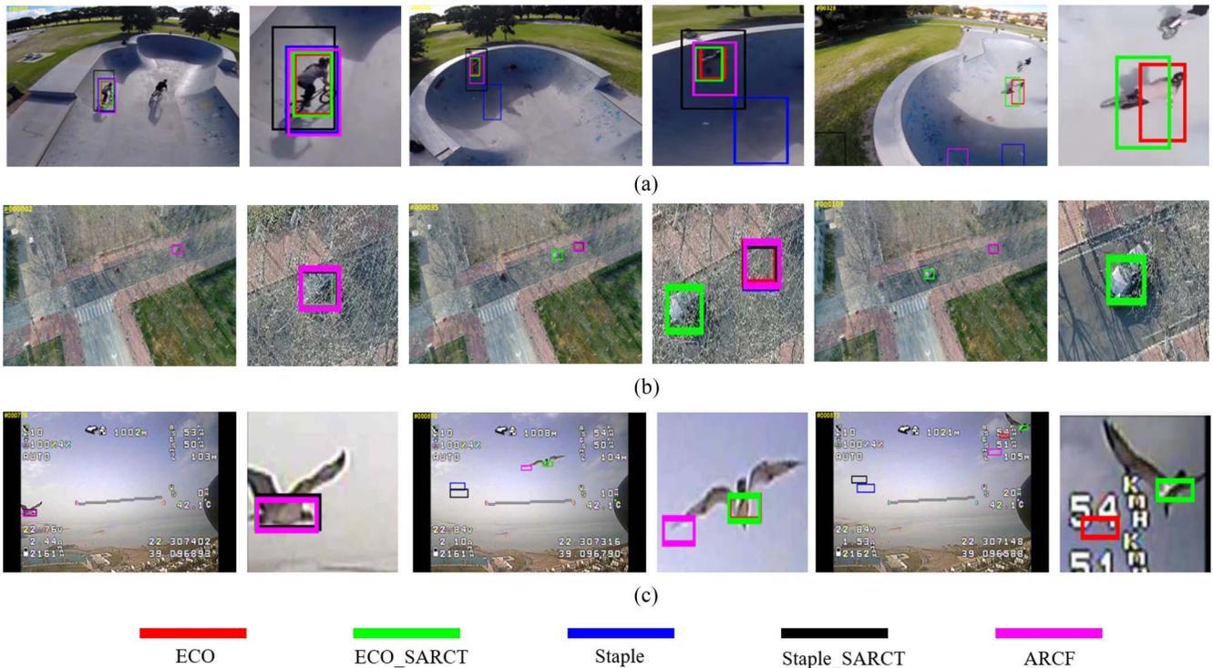
Fig. 7. Qualitative demonstration of the proposed ECO\_SARCT, Staple\_SARCT, their baselines, and the representative aerial tracker ARCF on sequences BMX4, S0103, and bird1 taken from DTB, UAVDT, and UAV123. (a) BMX4. (b) S0103. (c) bird1.
