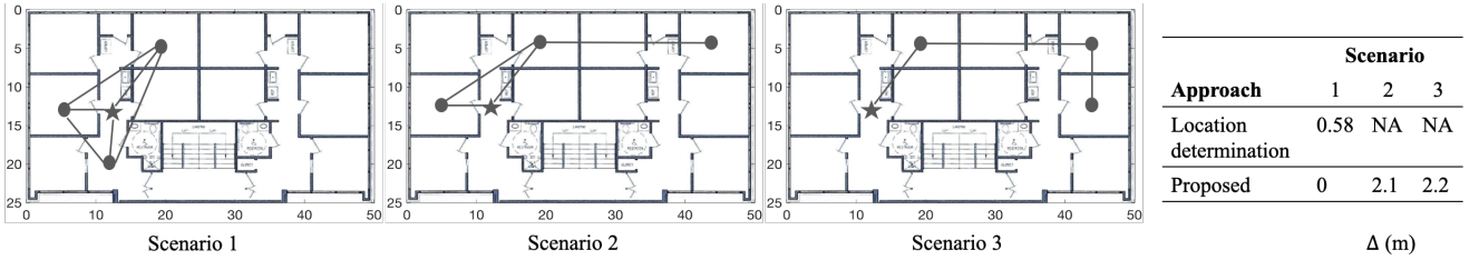
Fig. 12. Comparison with location determination based approach. Star represents the issuer AP, circles represent neighboring APs, and a solid line between two APs means that these are in coverage range of each other. Location determination (Trilateration) based approach can only detect geo-tampering in Scenario 1, where all 4 APs are in each other's coverage range. Our approach is applicable in all three scenarios.
