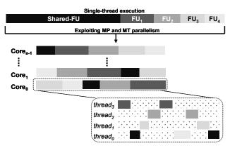
Figure 1: Exploiting MP and MT parallelism in the execution of the test program
