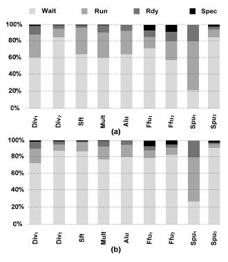
Figure 4: Test program profiling: exclusive single-thread execution for (a) manufacturing testing (b) post-silicon validation
