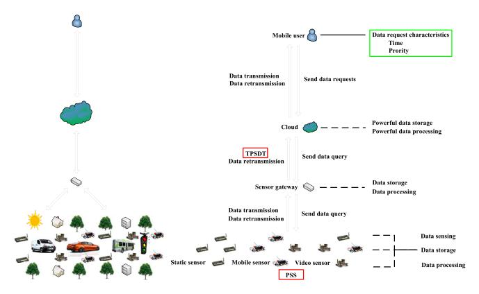
FIGURE 2. Proposed TPSS scheme to gather and transmit sensory data for WSN-MCC integration.
