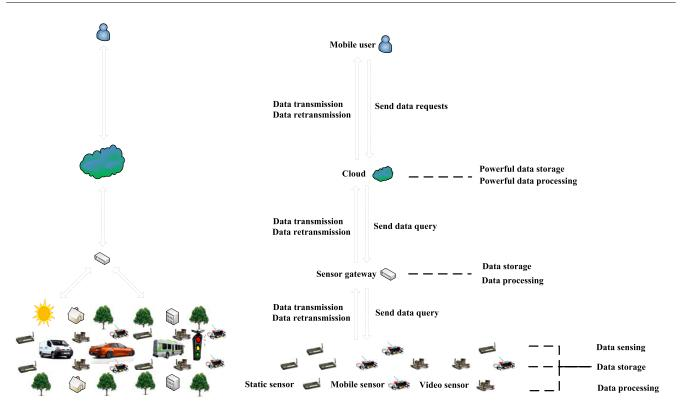
FIGURE 1. General scheme (GS) to gather and transmit sensory data for WSN-MCC integration.
