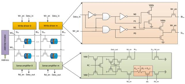
Fig. 12. Simulation circuits consisting of 1T-1MTJ array and peripheral circuits.
