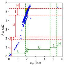
Fig. 9. Measured resistance distribution of  $R_P$  and  $R_{AP}$  for  $\not\!\!\!\!/ 60\,nm$  MTJ devices, suggesting the existence of states 'L', '0', 'U', '1', and 'H'.
