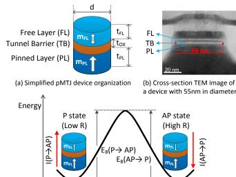
Angle between  $\mathbf{m}_{FL}$  and  $\mathbf{m}_{PL}(\theta)$ (c) Energy barrier between P and AP states
