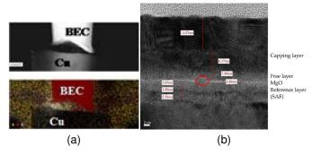
Fig. 5. TEM images of manufacturing defects: (a) an open contact defect between the BEC and the underlying Cu layer (reprinted from [27]), and (b) a pinhole defect in the MgO tunnel barrier of the MTJ device (reprinted from [36]).
