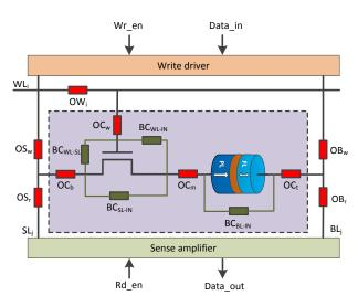
Fig. 6. Resistive defects in a single 1T-1MTJ memory cell.
