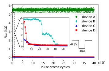
Fig. 14. The  $R_{\rm AP}$  of devices with pinhole defects degrades under pulse stress with elevated voltage and prolonged pulse width.
