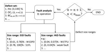
Fig. 11. Fault analysis methodology.
