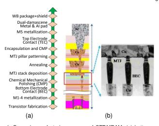
Fig. 4. General manufacturing process of STT-MRAM: (a) bottom-up processing flow of STT-MRAM cells, (b) vertical cross-section structure of STT-MRAM cells [27].
