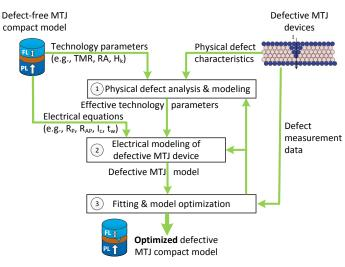
Fig. 7. Generic defect modeling flow.
