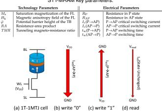
Fig. 3. Write and read operations of 1T-1MTJ cell.
