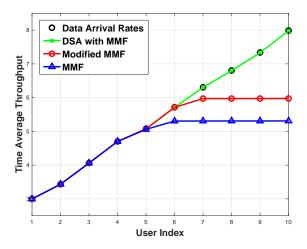
Fig. 5. Time-average throughput of K = 10 users with ZF processing in co-located Massive MIMO.  $B_{\text{max}} = 10 \times \tau_c$ ,  $p_1 = 0.3$ ,  $p_{10} = 0.8$ , uniform spacing between  $p_k$  and  $p_{k+1}$  for all  $k = 1, \ldots, 9$ .
