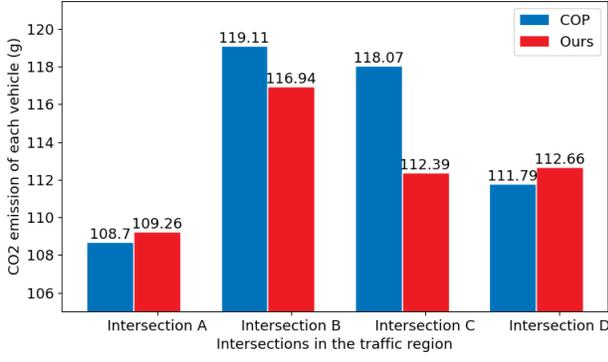
Fig. 8: The CO<sub>2</sub> emission comparison of our method and the COP algorithm. The x-axis is the intersection denoted as A, B, C, D. The y-axis is the average of CO<sub>2</sub> emission in 60-minutes simulation for each vehicle.
