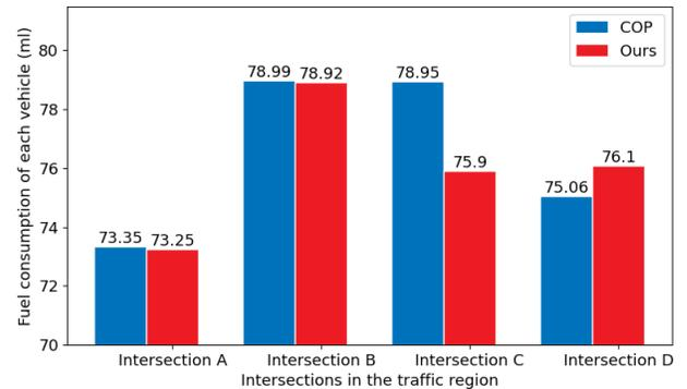
Fig. 7: The fuel consumption comparison of our method and the COP algorithm. The x-axis is the intersection denoted as A, B, C, D. The y-axis is the average of fuel consumption in 60-minutes simulation for each vehicle.
