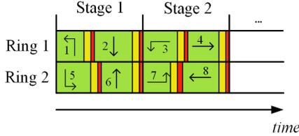
Fig. 3: Illustration of a signal plan for 8 phases.
