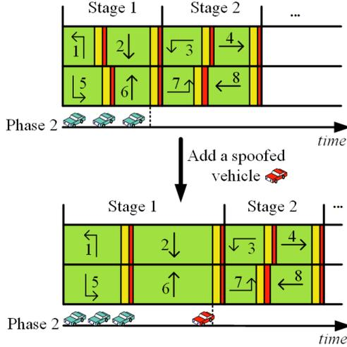
Fig. 9: Attack strategy of the 'last vehicle'. As shown, the spoofing vehicle was set on the phase 2, and in the end prolonged the green light duration of phase 2.
