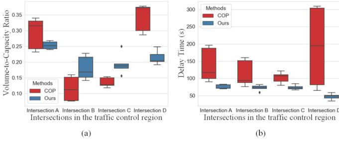
Fig. 5: Volume-to-Capacity Ratio ( $V/C$ ) and Delay Time ( $DT$ ) under normal traffic condition after 60-minutes simulation. The x-axis of (a) and (b) is the intersection denoted as A, B, C, D. The y-axis of (a) is the Volume-to-Capacity Ratio ( $V/C$ ), y-axis of (b) is the Delay Time ( $DT$ )(seconds).
