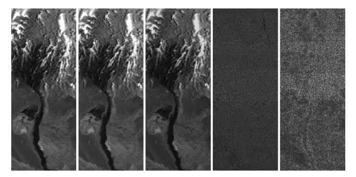
Fig. 6. Visual comparison of a crop of vgt1\_1b, band 1. From left to right: original image, predictive approach, transform approach, absolute error for predictive, absolute error for transform
