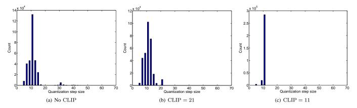
Fig. 3. AVIRIS sc0\_raw. (a) rate= 3.0052 bpp, MAD=30, SNR=62.25 dB; (b) rate= 3.0046 bpp, MAD=10, SNR=62.85 dB; (c) rate= 2.9968 bpp, MAD=5, SNR=63.39 dB
