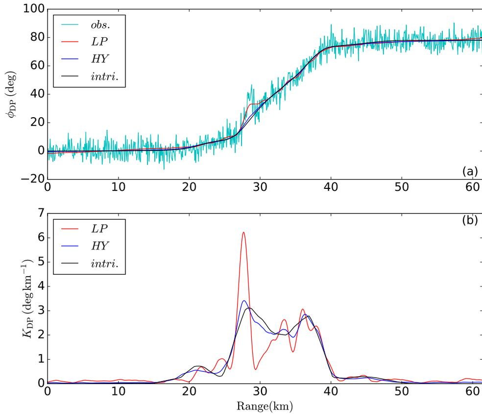
Figure 6: Comparisons of  $\phi_{DP}$  (a)/  $K_{DP}$  (b) estimates from the hybrid (blue solid) and basic linear programming (red solid) methods. Simulated  $\Phi_{DP}$  observations are denoted as cyan solid line in (a). The intrinsic  $\phi_{DP} / K_{DP}$  values are denoted with black solid lines.
