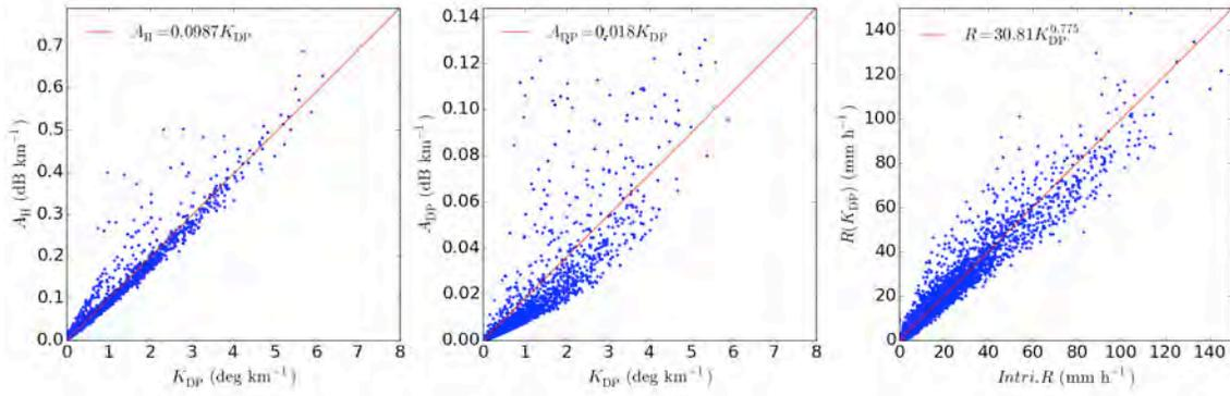
Figure 4: Specific attenuation ( $A_H$ : left) and specific differential attenuation ( $A_{DP}$ : middle) versus specific differential phase ( $K_{DP}$ ) for C-band, as well as the calculated intrinsic rainrate versus that estimated from  $K_{DP}$ .
