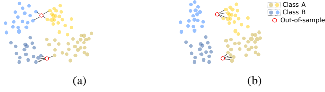
Fig. 2. Graphical illustration of the main limitation of SNCA. (a) In the metric space produced by SNCA, it will be challenging for the K NN classifier to distinguish the out-of-sample images located near the border between the two classes. (b) By introducing CE loss, these two classes are further separated in the metric space, and the same out-of-sample images in (a) can be accurately categorized by the K NN classifier.
