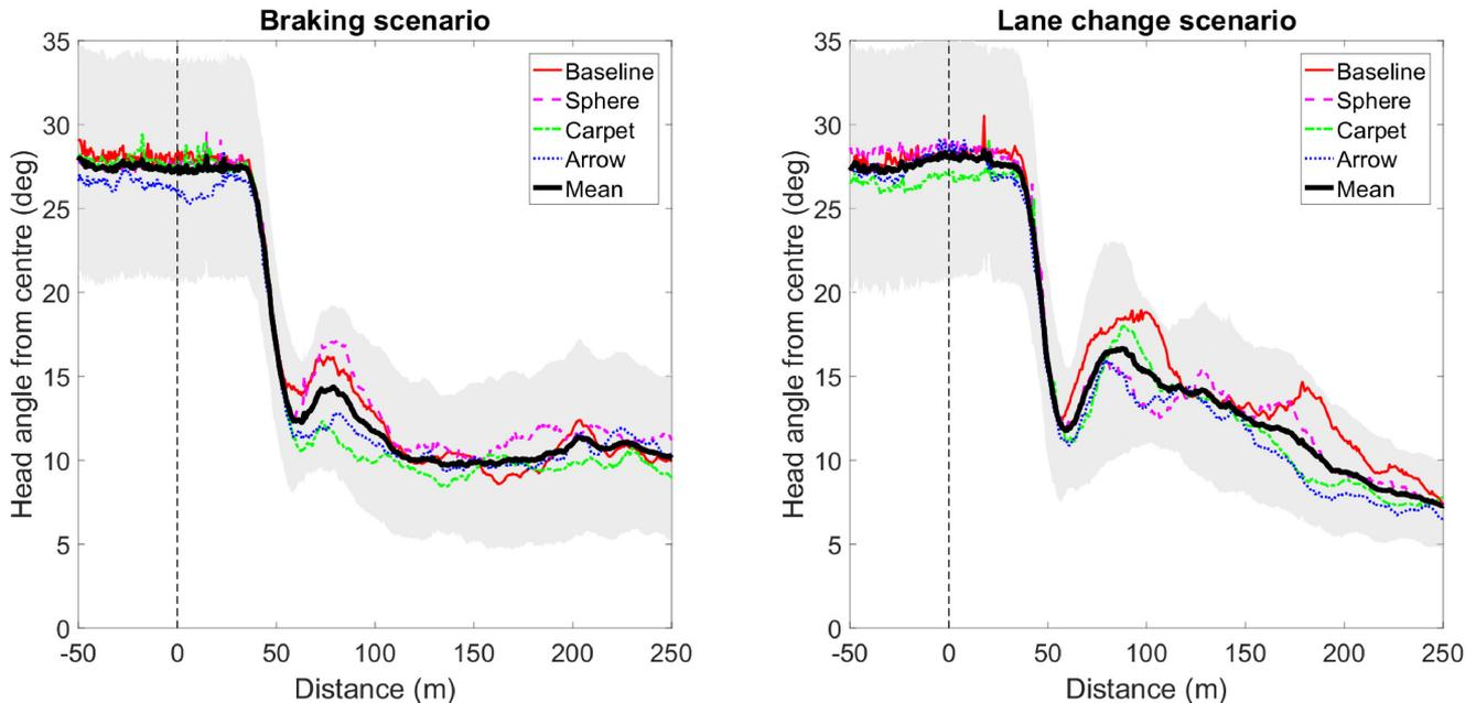
Fig. 5. Mean head angle across participants ( $N = 25$ ) as a function of travelled distance for braking (left) and lane change (right) scenarios. The shaded area around the (black) mean indicates the standard deviation across the means of the participants in all conditions. The vertical dashed line indicates the moment of the TOR.
