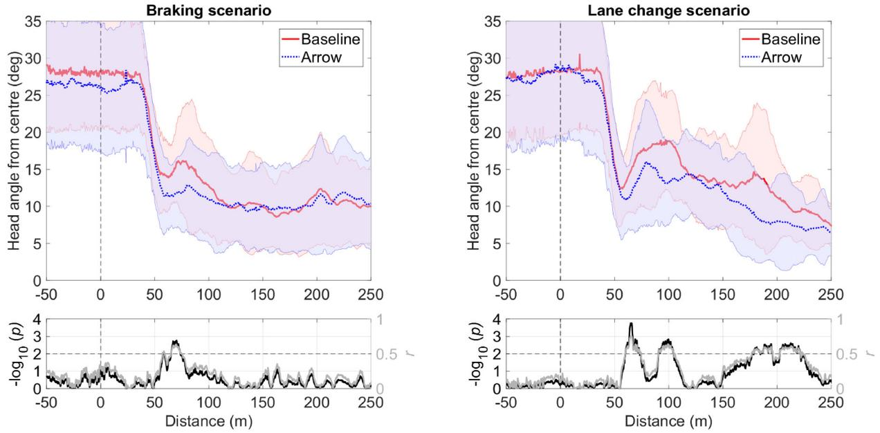
Fig. 6. Top: Mean and standard deviation (shaded area) of head angle across participants ( $N = 25$ ) as a function of travelled distance for the baseline and arrow conditions. The vertical dashed line indicates the moment of the TOR. Bottom:  $p$ -values from Wilcoxon signed-rank tests for the head angle between the baseline and arrow conditions. The horizontal dashed line indicates a threshold of  $p = 0.01$ .
